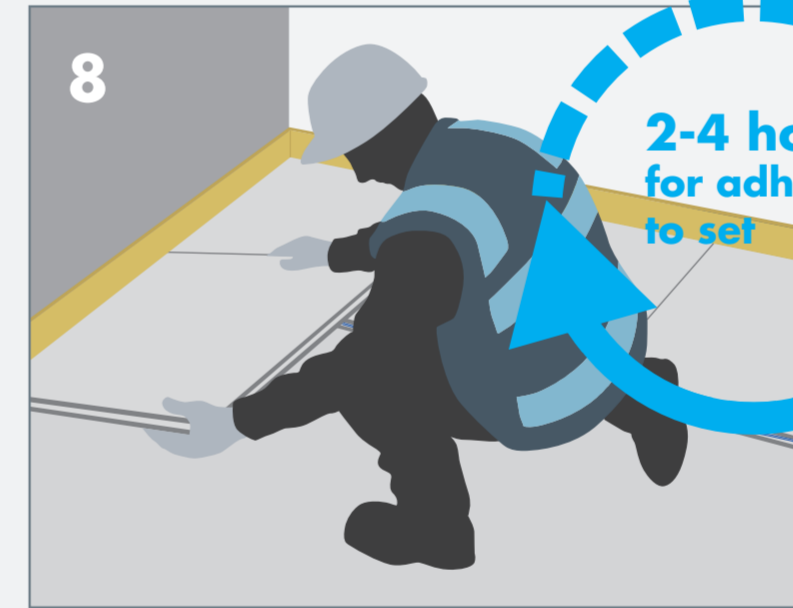
8 Cut off from first row starts the next (minimum 200mm overlap).
