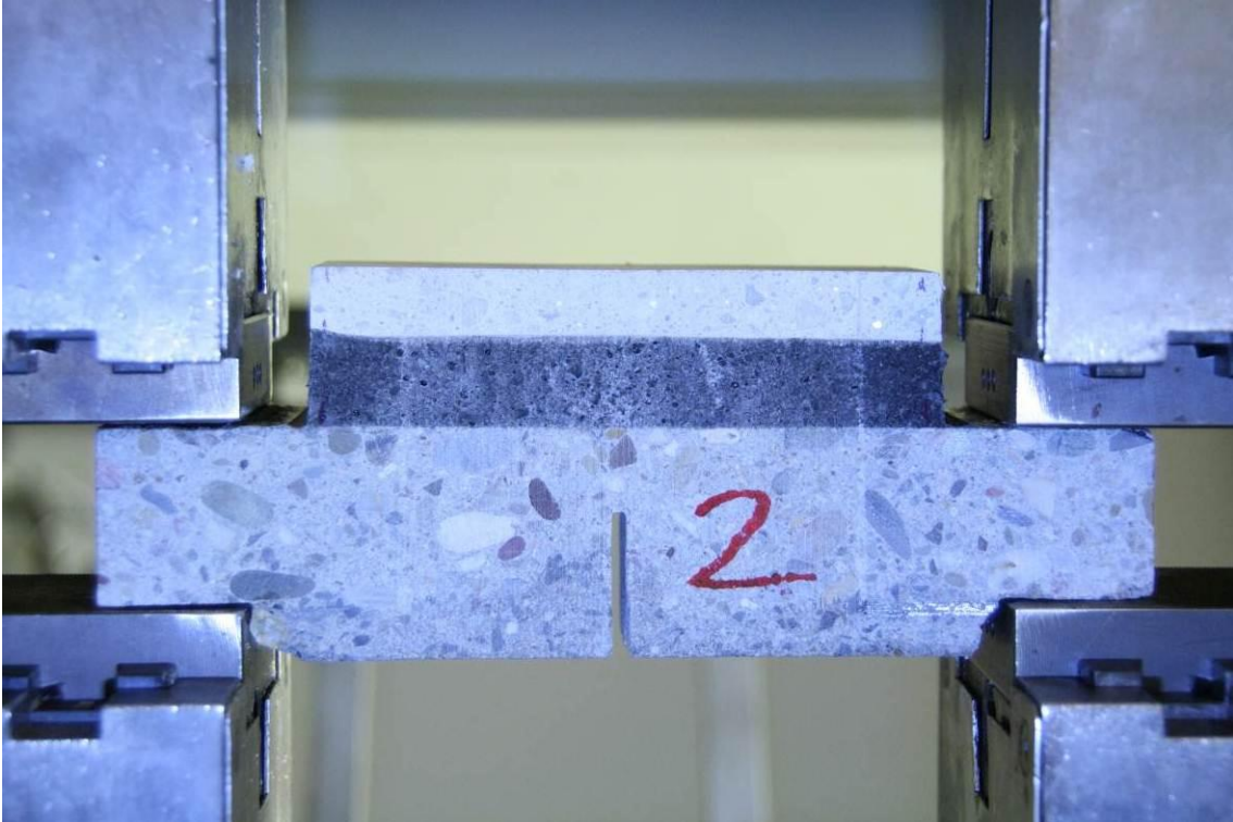
Photo 2, Start position of a test, with cut in the concrete.
