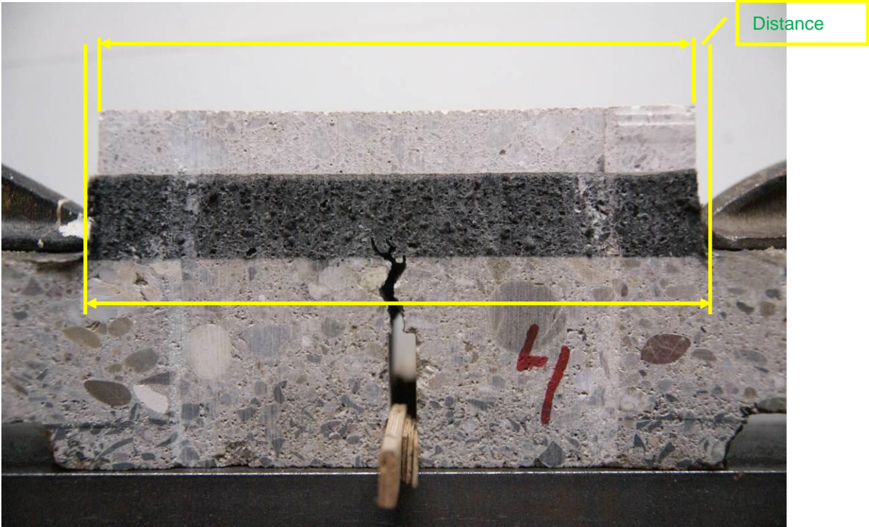
Photo 6, Lasting crack bridging over a crack of 2.6 mm wide.
