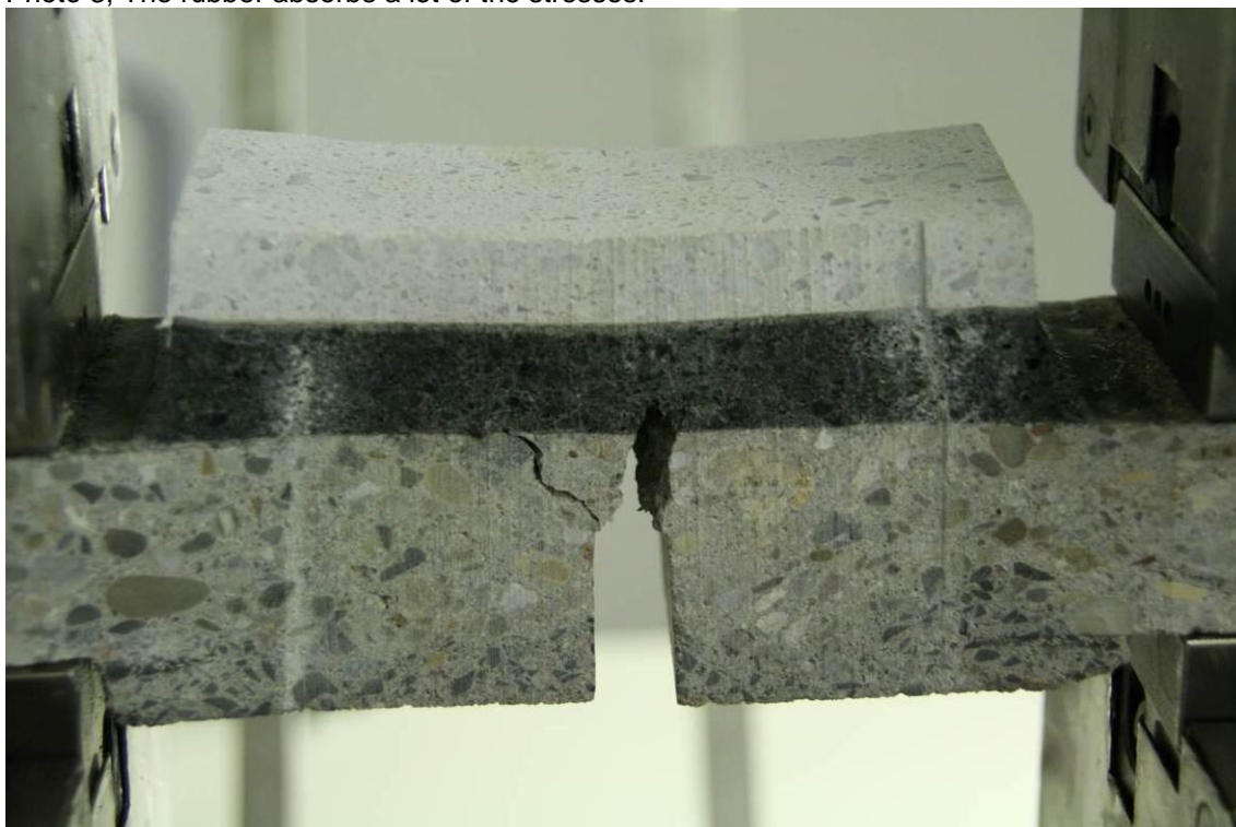
Photo 4, At a certain point the rubber starts to tear. Deformation is visible on sample surface.
