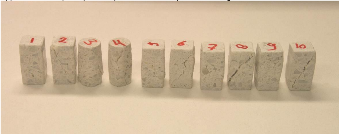
Photo 1, Samples upon completion of the compression strength test.
