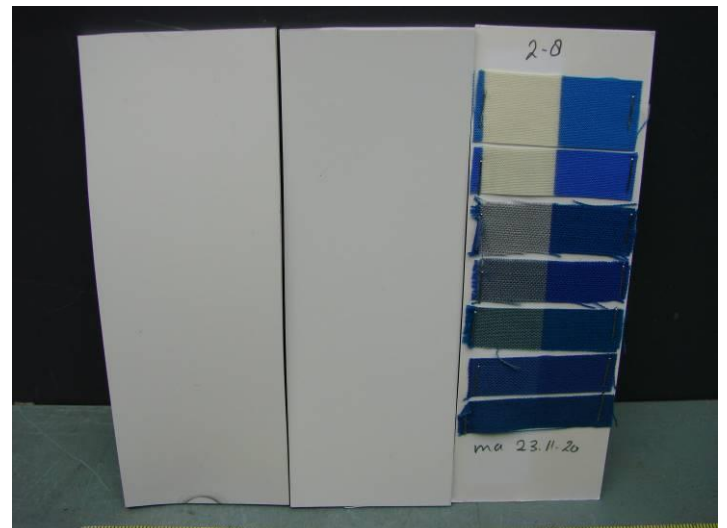
Photo 5: Xenotest, 1500 hours. Test panel on left side.
