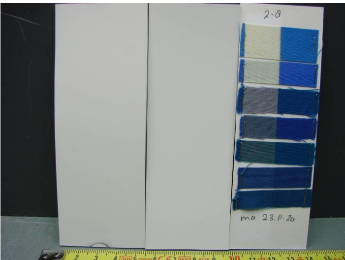
Photo 4: Xenotest, 1002 hours. Test panel on left side.
